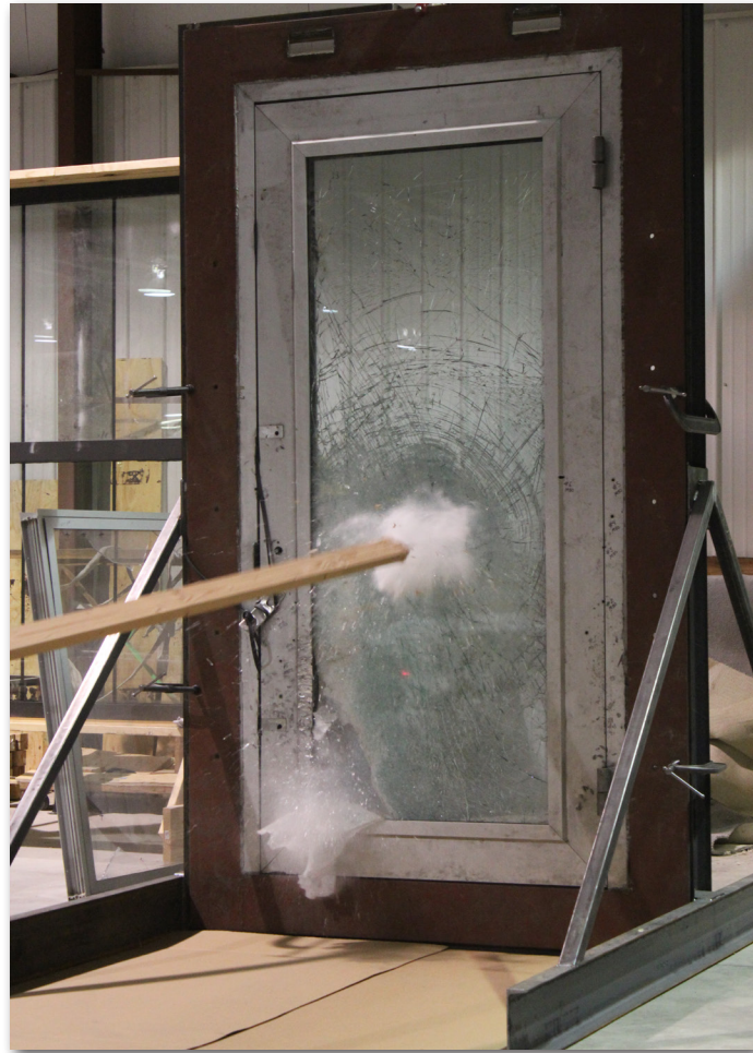
Winco tornado and impact testing: Winco architectural-grade pre-glazed windows, incorporating Tremco's Spectrem 2 Silicone Sealant and 440 Tape, were tested for tornado and impact resistance.
